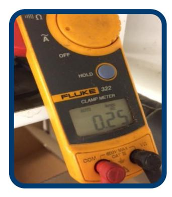
3 x EC motors with new Carbon Fiber blades amp draw 0.25 amps
