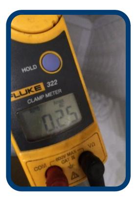
3 x EC motors with new Carbon Fiber blades amp draw 0.25 amps
