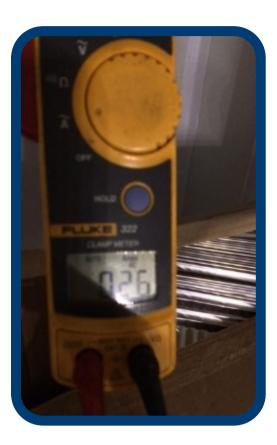
3 x EC motors with new Carbon Fiber blades amp draw 0.26 amps
